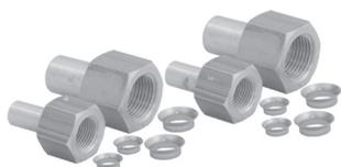
Alternatively, the refrigerant lines can also be connected using the Euro flanged adaptor connection kit for hard-soldering on refrigerant lines (lines must be flushed with nitrogen), available from the WOLF range of accessories.
