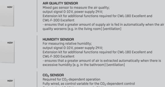
Fully wired, as control variable for the CO<sub>2</sub>-dependent control Output signal 0-10 V, power supply 24 V Extension kit for additional functions required for CWL-180 Excellent and CWL-F-300 Excellent - ensures that a greater amount of supply air is fed in automatically when the CO<sub>2</sub> content is excessive
